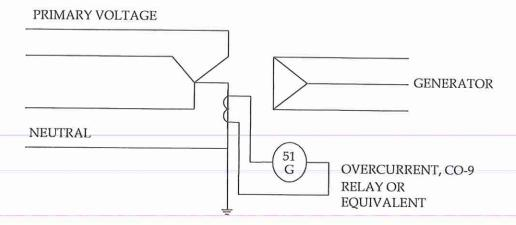
The system below illustrates a distribution system with the service transformer connected delta on the primary voltage side.
